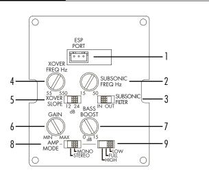
NOTE: The adjustment for Gain is a digital control (potentiometer). Although it will have the feel of adjustment like the other controls on this panel (there are no detents), the Gain control has 33 discrete steps in adjustment. Hence a small rotational change in the Gain adjustment may not affect the gain of the amplifier.
